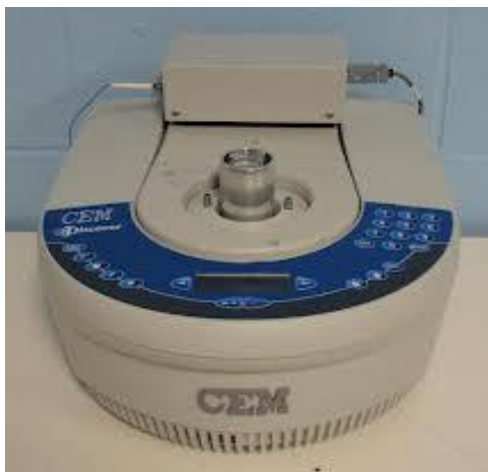
Figure 6. Focused mono-mode microwave oven (CEM corporation, Matthews, NC)
