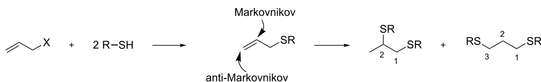
Scheme 1: Sequential substitution-addition reactions of thiols with allyl halides leading to the formation of 1,2 or 1,3-dithioethers.
