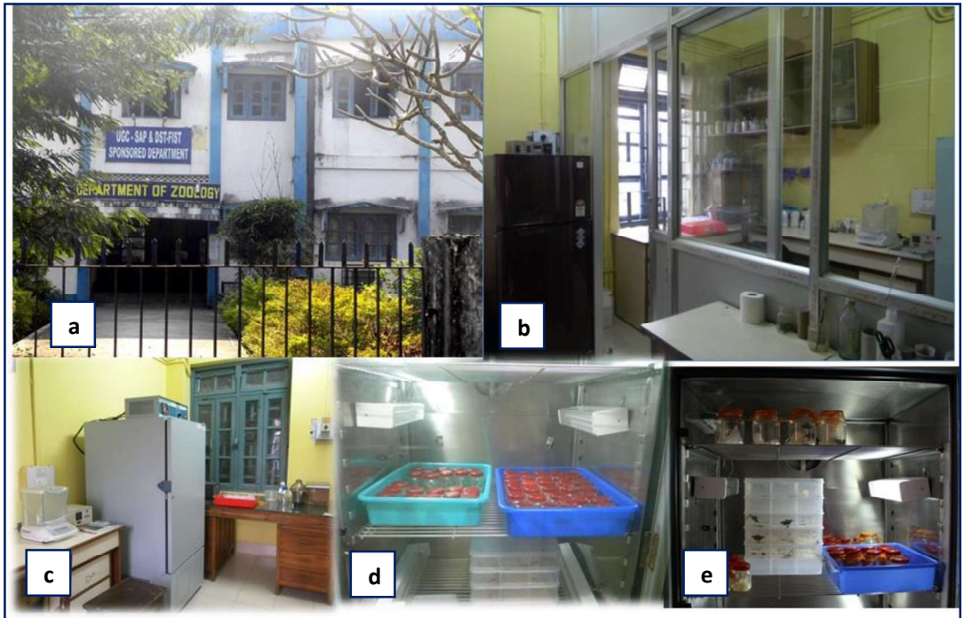
Figure 5.6.1 Laboratory set up for insect-rearing at Department of Zoology [insets: (a) Front elevation of Zoology Department, (b) Ante chamber for the rearing room, (c) Inner view of rearing cubicle within glass partition, (d) Rearing trays inside BOD incubator, (e) Set up inside BOD incubator for group and individual rearing]
