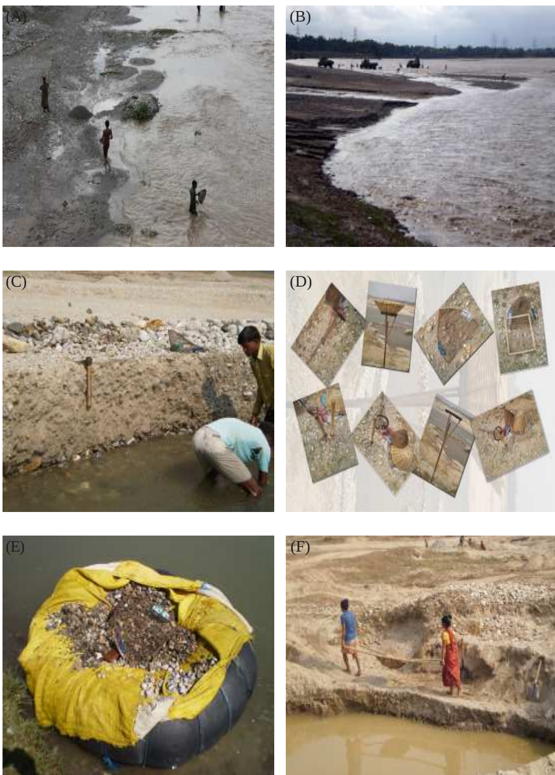
Plate 5.3 The extraction activities during monsoon periods (A & B); cutting of river bed for extracting better quality materials (C); the tools used for extraction process (D, E & F).
