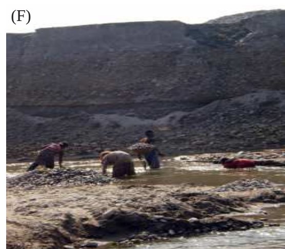
Plate 6.2 Direct extraction from active channel flow by extractors causing bed erosion (A); tree trunks (red circled) being exposed due to prolonged extraction causing incision (B, C, D & E); and near bank extraction diverting channel flow (F) in the lower Balason river.
