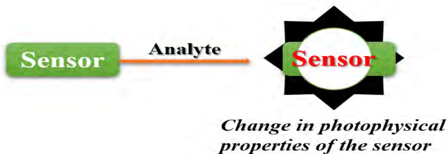
Figure-1.3. A diagram illustrating a sensor that undergoes alterations in its photophysical properties upon detecting an analyte.
