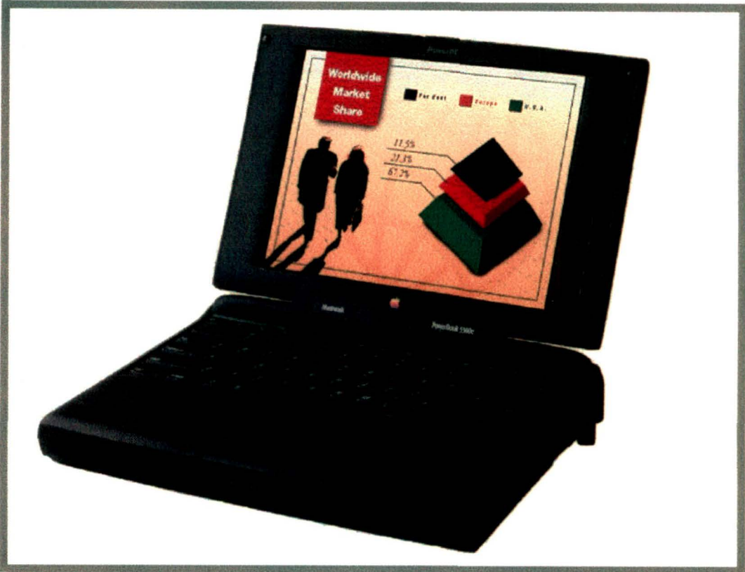
Plate 2 Portable computer with an active matrix colour liquid crystal display.
