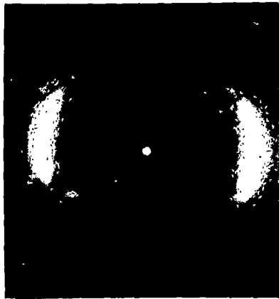
Figure 6.7 : X-ray diffraction photograph of oriented sample 1d(3)CC at 60°C.
