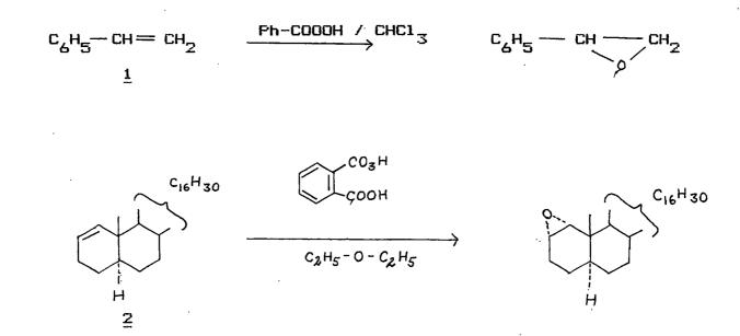
Carbon-Carbon double bond is selectively oxidised 3 (eg.3 ) in presence of hydroxyl or carbonyl functions.
