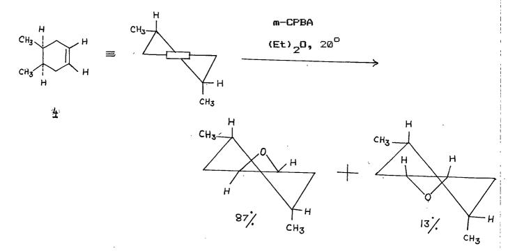
The use of perbenzoic acid or mCPBA in chloroform or methylene chloride has an advantage of isolating the epoxide formed while epoxidation reactions with olefin 5 run with peracids in presence of an excess of the corresponding carboxylic acid frequently yield the hydroxy esters<sup>5</sup> derived from the initially formed epoxide.
