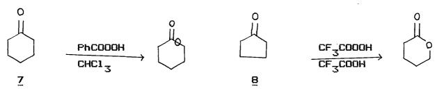
The conversion is catalysed by acids and the rate of oxidation is accelerated by electron donating groups in the ketone and electron withdrawing groups in the per acids.
