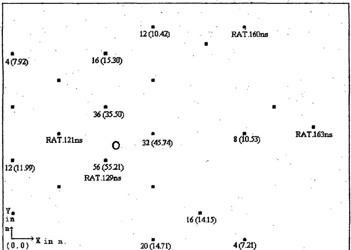
Fig.3.1b: Observed EAS event and reconstructed shower parameters from that data.
