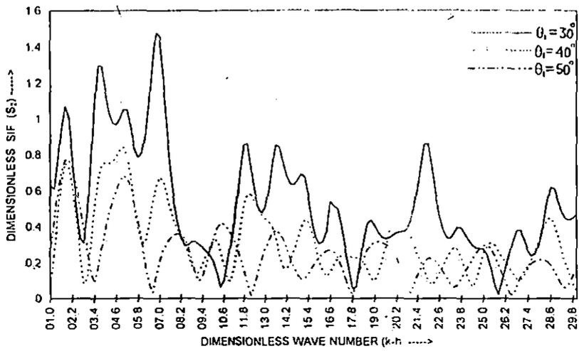
Fig.6 Stress intensity factor  $S_2$  versus dimensionless wave number  $k_1h$  for  $\theta_1=30^\circ$ ,  $40^\circ$ , and  $50^\circ$ .
