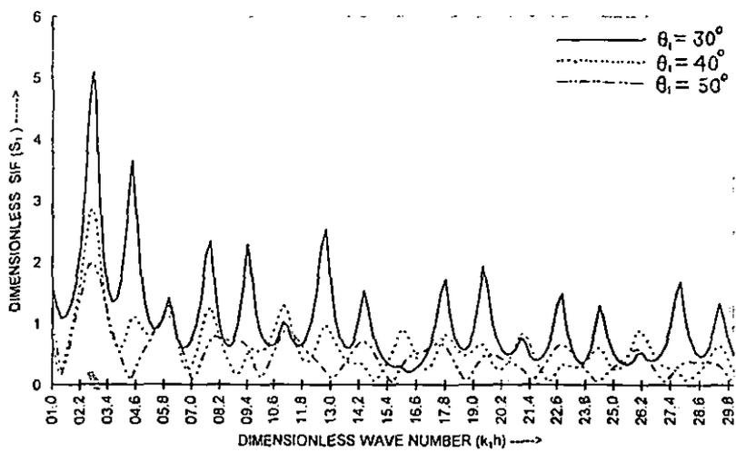
Fig.5 Stress intensity factor  $S_I$  versus dimensionless wave number  $k_1h$  for  $\theta_1=30^\circ$ ,  $40^\circ$ , and  $50^\circ$ .
