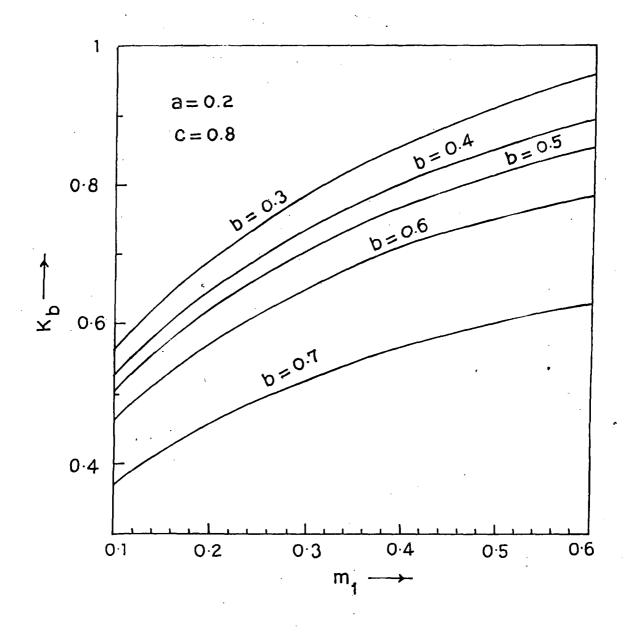
Fig. 7. Stress intensity factor  $K_b$  versus dimensionless frequency m<sub>1</sub> for a = 0.2, c = 0.8 and for different values of b.
