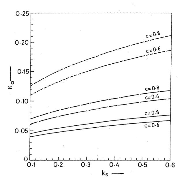
Fig. 6. Stress intensity factor  $K_a$  vs. frequency  $k_s$  for generalized plane stress.
