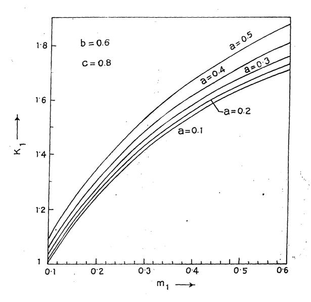
Fig. 5. Stress intensity factor  $K_1$  versus dimensionless frequency  $m_1$  for b = 0.6, c = 0.8 and for different values of a.
