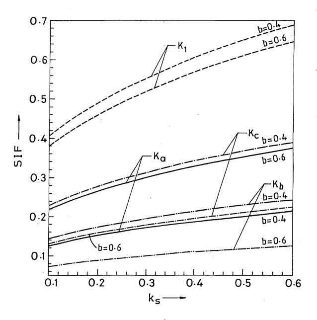
Fig. 4. Stress intensity factors vs. frequency k for generalized plane stress.
