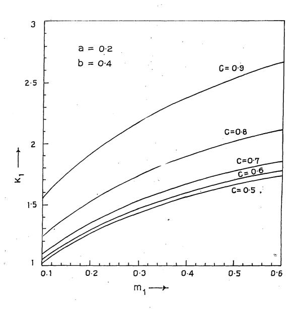
Fig. 13. Stress intensity factor  $K_1$  versus dimensionless frequency  $m_1$  for a = 0.2, b = 0.4 and for different values of c.
