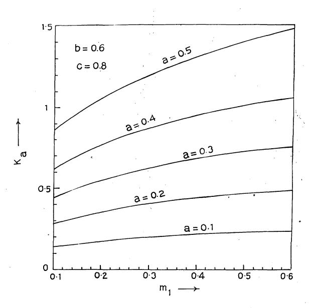
Fig. 2. Stress intensity factor  $K_a$  versus dimensionless frequency  $m_1$  for b = 0.6, c = 0.8 and for different values of a.
