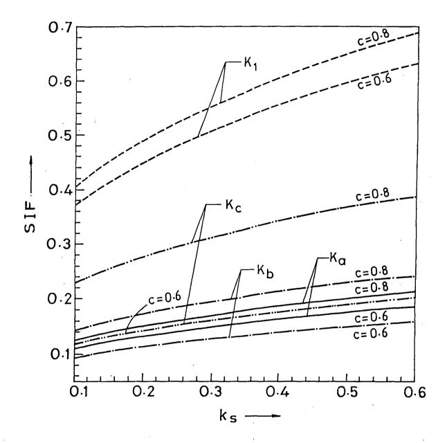
Fig. 5. Stress intensity factors vs. frequency k for s
