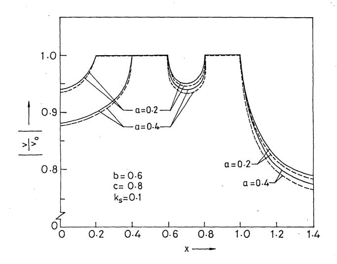
Fig. 7. Vertical displacement  $| v/v_0 |$  vs. distance x for generalized plane stress.
