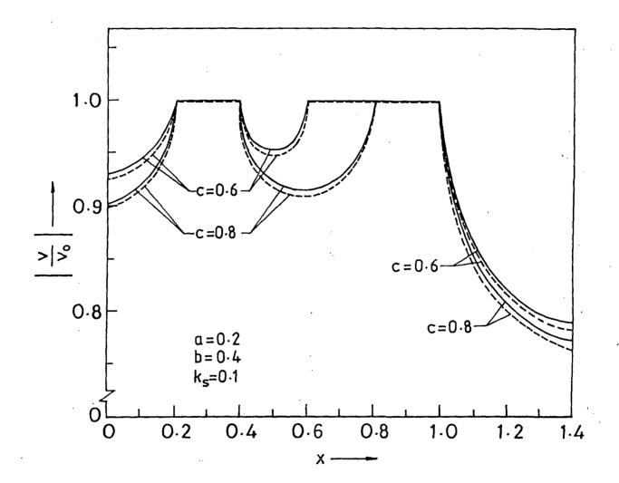
Fig. 9. Vertical displacement | v/v<sub>0</sub> | vs. distance x for generalized plane stress. ( ----- Type I, ----- Type II ).
