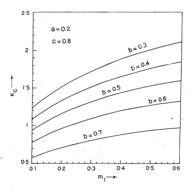
Fig. 8. Stress intensity factor K versus dimensionless frequency m for a = 0.2, c = 0.8 and for different values of b.
