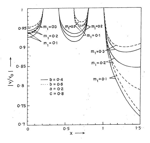
Fig. 15. Vertical displacement  $| v(x,0)/v_0 |$  versus dimensionless distance x for a = 0.2, c = 0.8, b = 0.4, 0.6 and for m<sub>1</sub> = 0.1, 0.2, 0.3.
