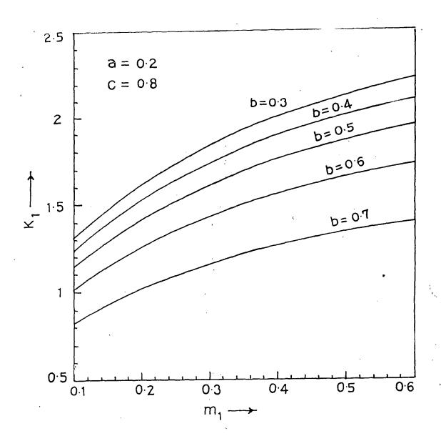
Fig. 9. Stress intensity factor  $K_1$  versus dimensionless frequency  $m_1$  for a = 0.2, c = 0.8 and for different values of b.
