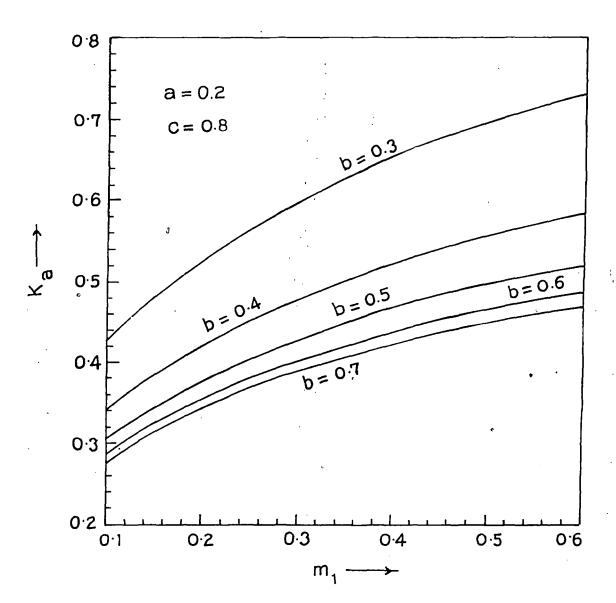
Fig. 6. Stress intensity factor  $K_a$  versus dimensionless frequency m<sub>1</sub> for a = 0.2, c = 0.8 and for different values of b.
