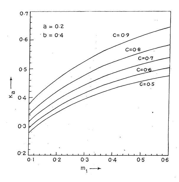
Fig. 10. Stress intensity factor K<sub>a</sub> versus dimensionless frequency  $m_1$  for a = 0.2, b = 0.4 and for different values of c.
