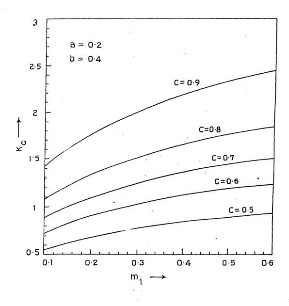
Fig. 12. Stress intensity factor K<sub>C</sub> versus dimensionless frequency  $m_1$  for a = 0.2, b = 0.4 and for different values of c.
