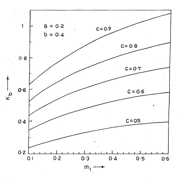
Fig. 11. Stress intensity factor K versus dimensionless frequency m<sub>1</sub> for a = 0.2, b = 0.4 and for different values of c.
