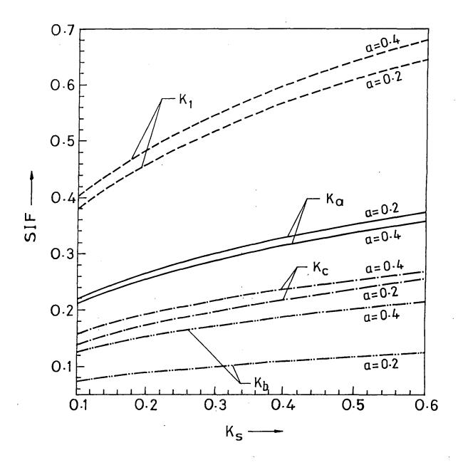
Fig. 3. Stress intensity factors vs. frequency k for generalized plane stress.
