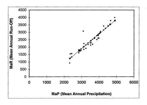
The correlation co-efficient between the mean annual precipitation (X) and the mean annual run-off (Y) is very high (r = 0.937) and have a 't' value of 14.155 which is significant at the level of 0.005 %. The regression equation is:
