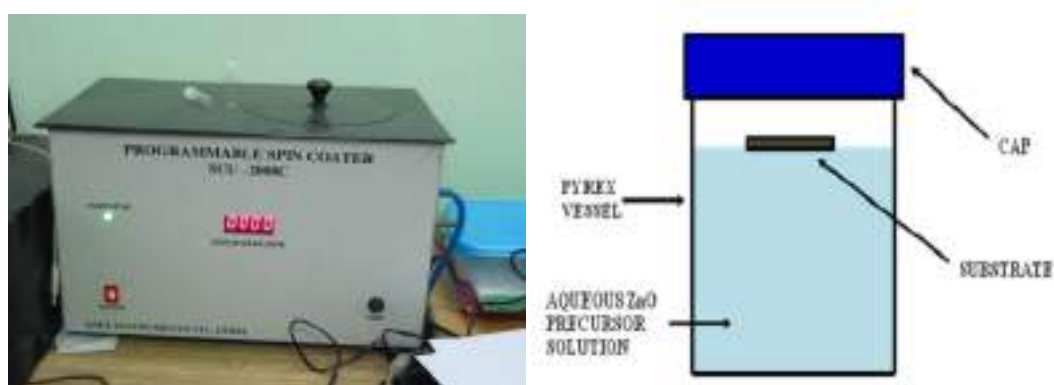
Figure 3.5 (a) Spin Coater for seed layer formation (b) vessel for nanorod grow.
