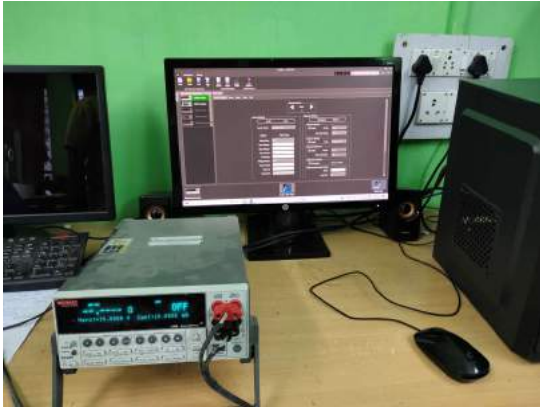
Figure 2.10 Experimental Setup for I-V measurement.
