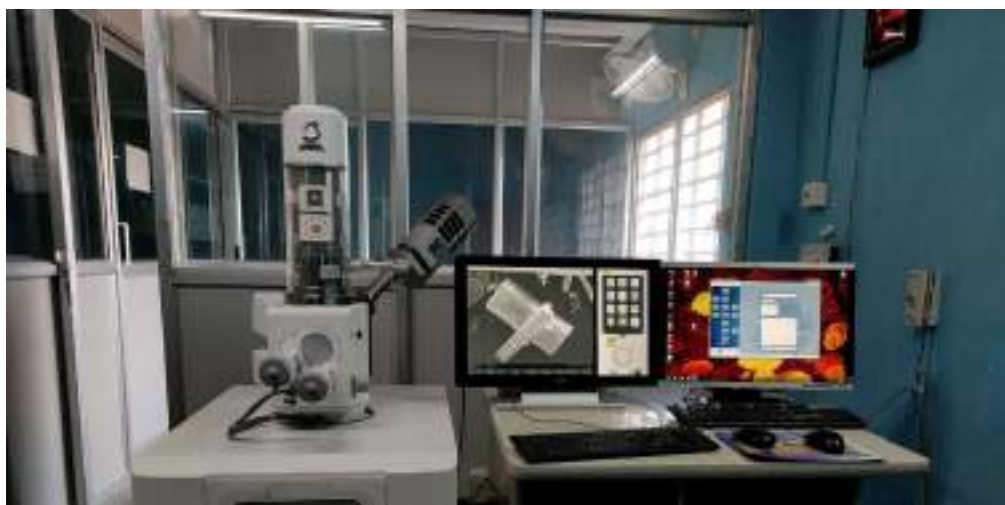
Figure 2.3 Experimental setup for SEM and EDS measurement.
