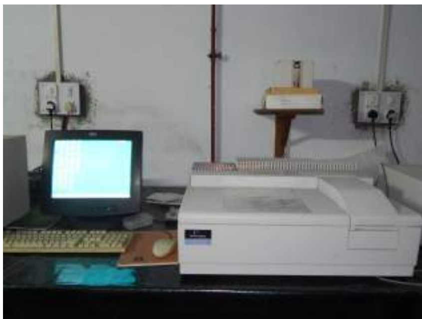
Figure 2.5 Experimental setup for UV-VIS absorption measurement.
