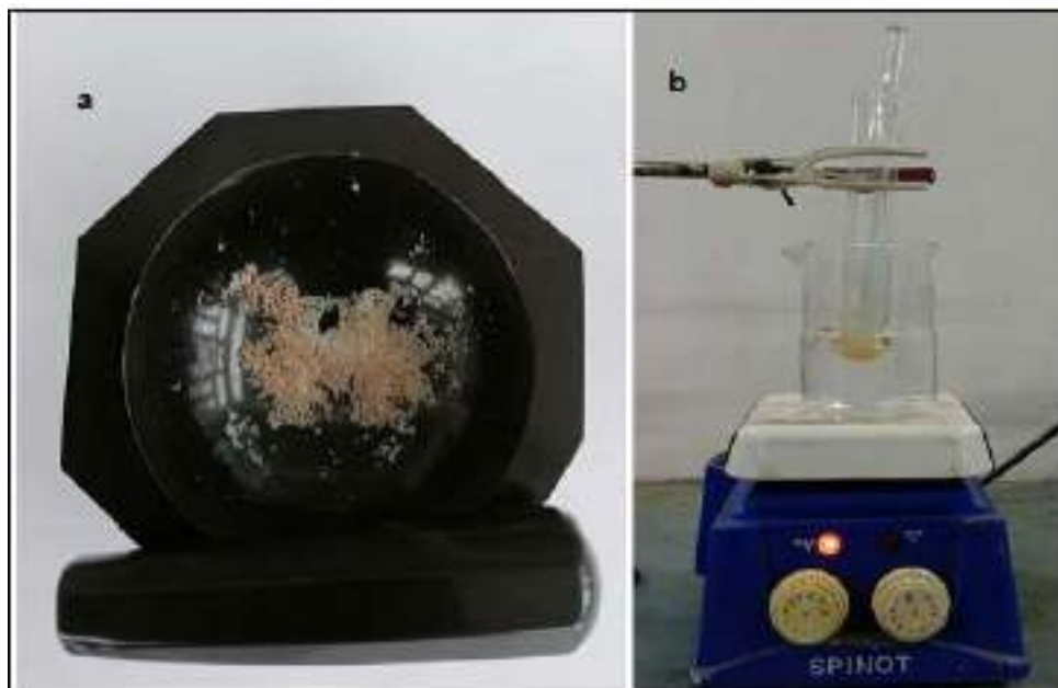
Fig. 2.1. a) Pulverization of reactant and catalyst in agate mortar and pestle and b) Heating the reaction mixture in oil bath.
