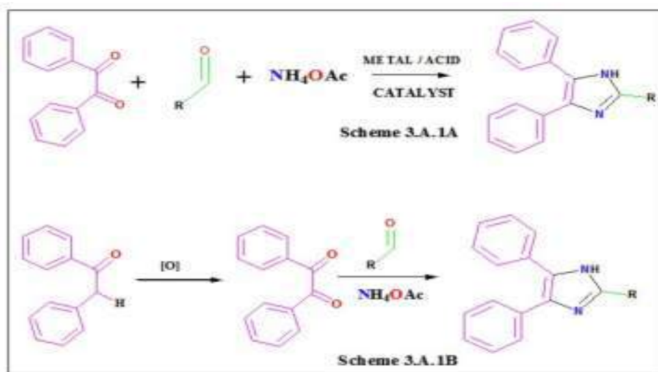
Scheme. 3.A.1A. Debus-Radiszewski imidazole synthesis and Scheme. 3.A.1B. Synthesis of tri-substituted imidazole using \alpha -hydroxyketone.
