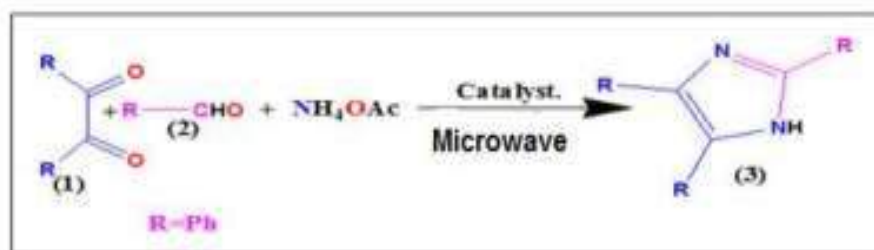
Scheme. 1.22. Synthesis of 2,4,5-triaryl imidazoles under microwave irradiation.
