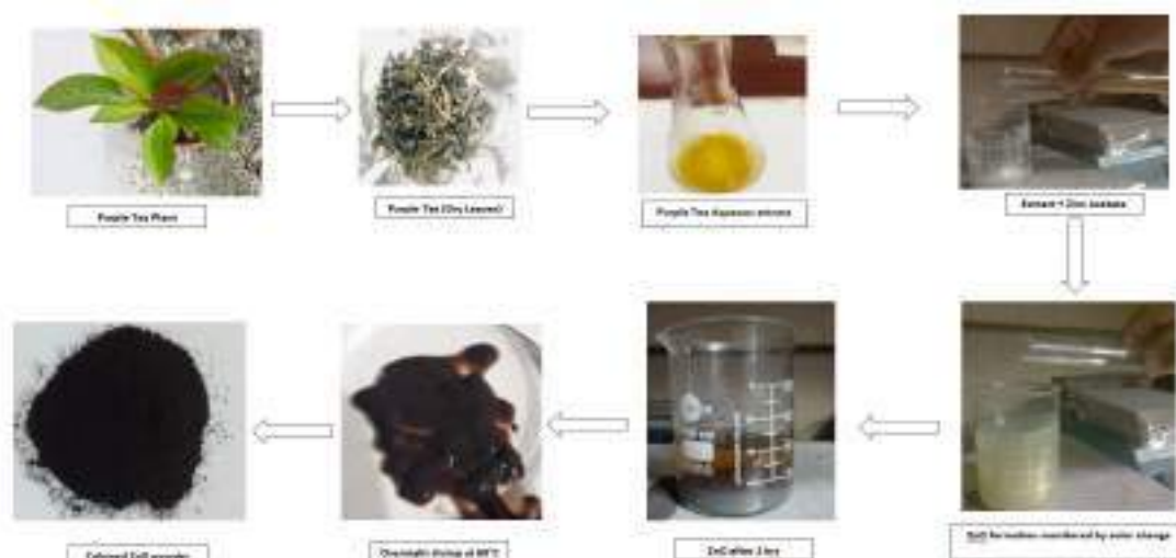
Fig.4.31. Schematic diagram of synthesis of Zinc Oxide nanoparticles (ZnO NPs) from purple tea extract
