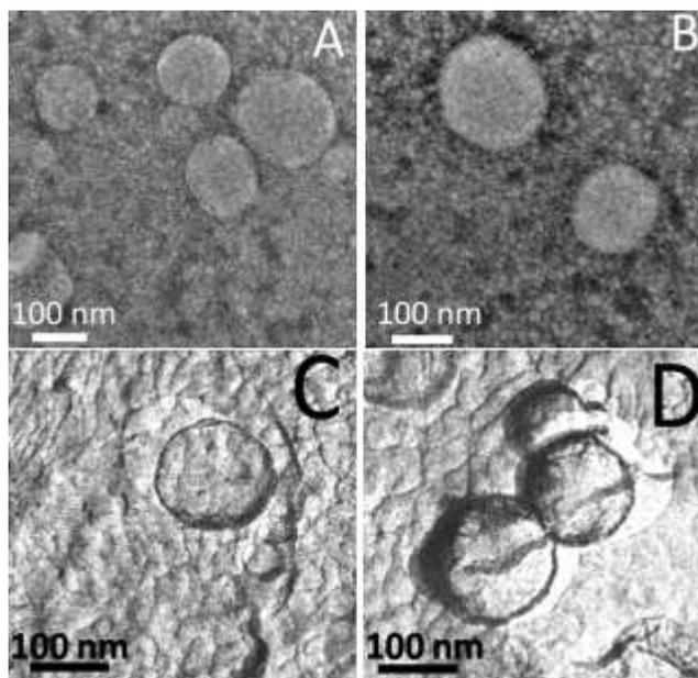
**Figure 6.** TEM (panel A, B) and FF-TEM (panel C, D) images for NLC (CP+TP+OA, 2:2:1, M/M/M) formulations in the absence (panel A, C) and presence (panel B, D) of chrysin. The scale bars are mentioned inside the figure.
