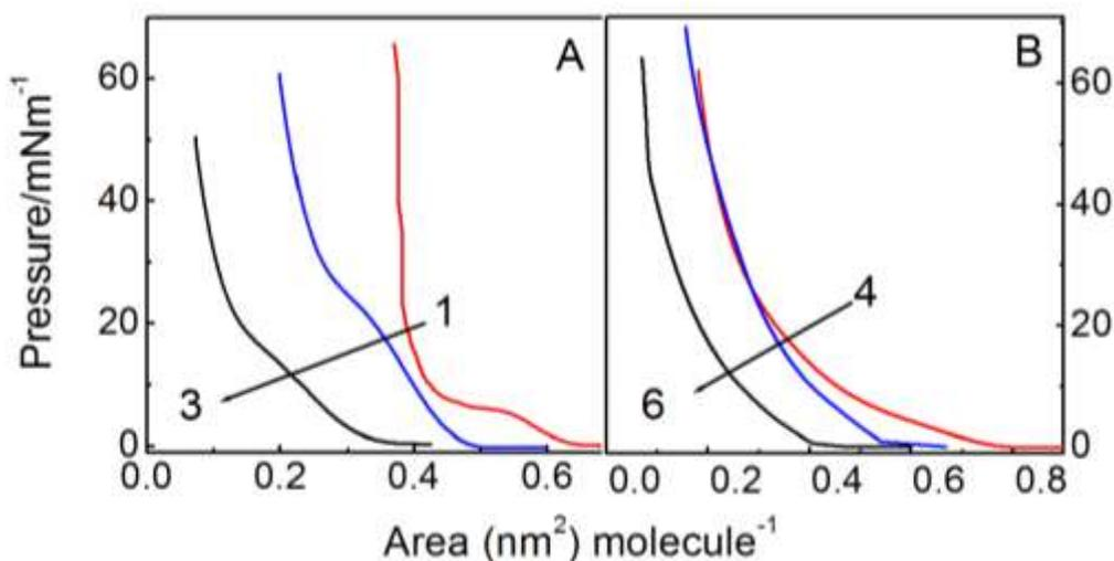
**Figure 1.** Surface pressure ( $\pi$ )- area (A) isotherms of pure lipids using water (panel A) and 2mM aqueous Tween 60 solution (panel B) as the subphase at 25°C. Systems: 1 & 4, TS; 2 & 5, OA; 3 & 6, CP.
