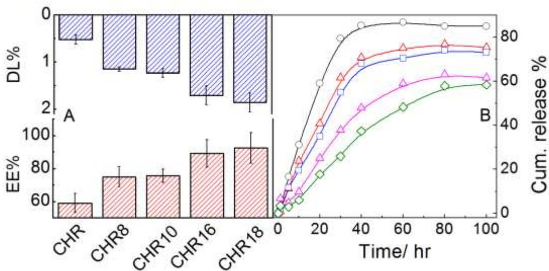
**Figure 11.** Entrapment efficiency (EE%), drug loading (DL%) capacity (panel A) and release profile (panel B) of chrysin and different LCDs of chrysin form NLC formulation at 25 °C . systems (panel B): O, CHR; Δ, CHR 8; □, CHR 10; ▽, CHR 16 and◇, CHR 18.
