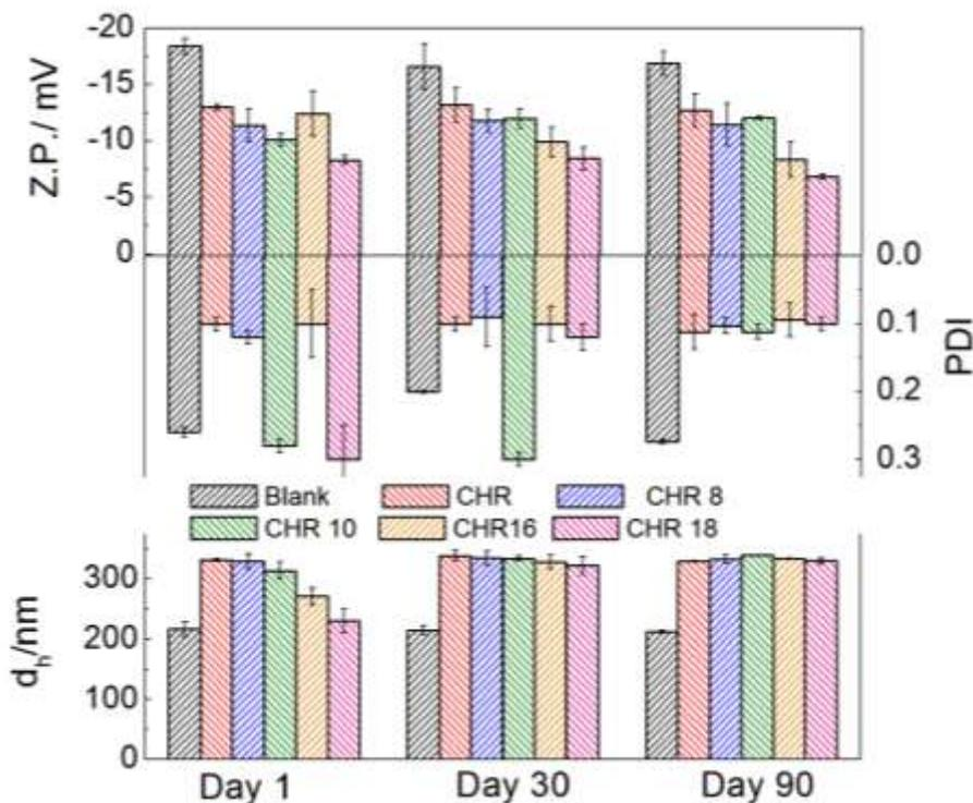
**Figure 5.** Variation of hydrodynamic diameter, PDI and zeta potential with time for 1 mM NLC formulation (CP+TP+OA, 2:2:1, M/M/M) stabilized by 2 mM aqueous Tween 60 solution in the absence and presence of chrysin and LCDs of chrysin at 25 °C. Individual systems are mentioned inside the figure. [Chrysin] & [LCDs of chrysin]: 10  $\mu$ M.
