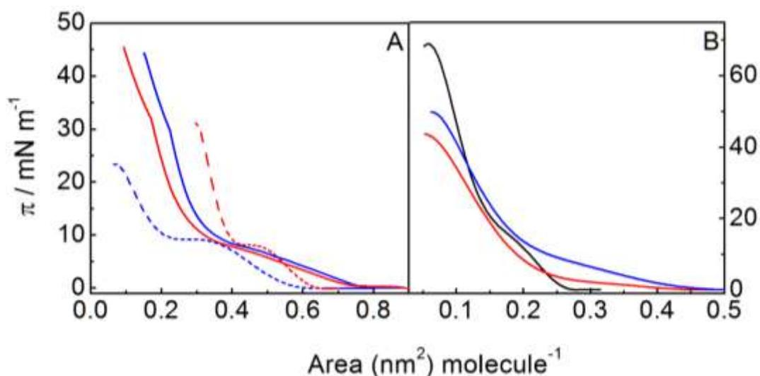
**Figure 2.** Surface pressure ( $\pi$ ) – area (A) isotherm of CHR 10 (blue) and CHR 16 (red) using water (dotted line) and 2 mM aqueous Tween 60 solution (solid line) as subphase (panel A). Panel B represented the  $\pi$  – A isotherms of mixed lipidic system (CP+TP+OA, 2:2:1, M/M/M) in absence (black) and presence of 50 mole% CHR 10 (blue) & CHR 16 (red) using 2mM aqueous Tween 60 as subphase. Temperature 25 °C.
