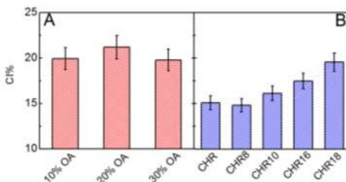
**Figure 10.** Crystallinity index (CI%) of the NLC formulations (CP+TP+OA, 2:2:1, M/M/M) in the absence (panel A) and the presence (panel B) of chrysin and LCDs of chrysin. The individual systems are mentioned in the figure.
