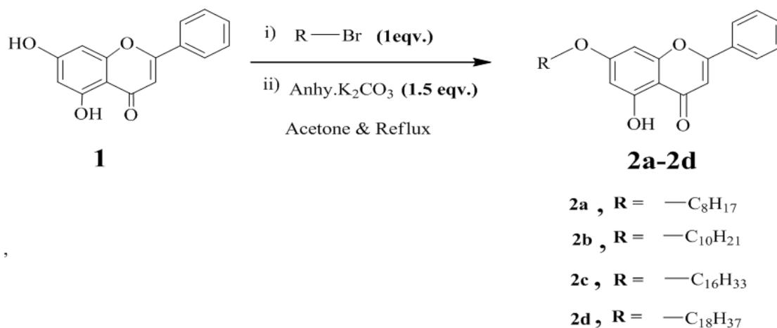
**Scheme 1.** Synthesis of C (7) modified derivatives (LCD's) of chrysin.
