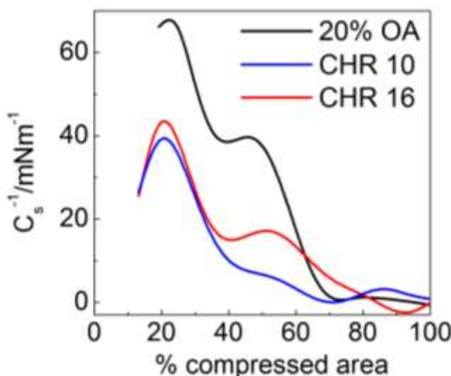
**Figure 3.** Variation of elasticity moduli ( $C_s^{-1}$ ) with % compressed area upon addition of 50 mole% different LCDs of chrysin on the mixed lipidic system (CP+TP+OA, 2:2:1 M/M/M). 2mM aqueous Tween 60 was used as subphase. Different systems have been mentioned inside the figure.
