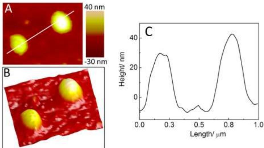
**Figure 7.** AFM image of NLC (CP+TP+OA, 2:2:1, M/M/M) formulation where panel A and B represented the two and three dimensional view respectively. Panel C represented the roughness profile for the NLC formulation. Height scale is given inside the figure. Scane area: (1X1)  $\mu\text{m}$ .
