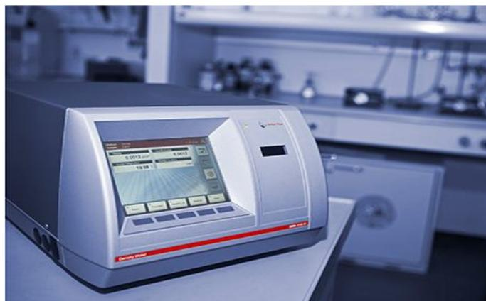
In the digital density meter, the mechanic oscillation of the U-tube is e.g. electromagnetically transformed into an alternating voltage of the same frequency. The period  $\tau$  can be obtained by the following relation with  $\rho$  of the sample in the oscillator [10]:
