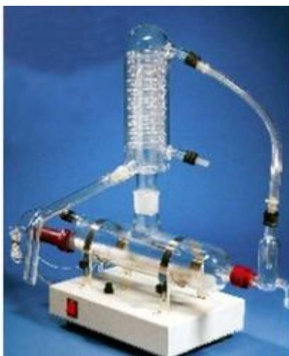
Water Distiller is usually made by the Borosil Glass material. A distilling solvent in the boiling chamber heats the water until it boils off. The vapour rises from the boiling chamber. Volatile contaminants are discharged through a built-in vent tube. Minerals and salts are retained in the boiling chamber as hard deposits. The steam passed into the condenser, which is condensed by cool water. Droplets of water poured into the collecting container.
