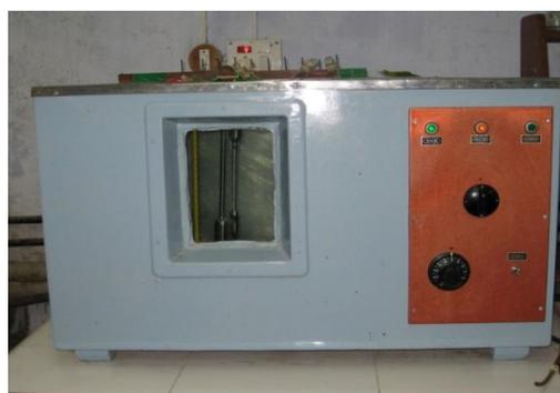
Laboratory water bath is a system in which a container containing water and the investigated solution is placed over this container to quickly heat. These laboratory equipments are available in different volumes and construction with both digital and analogue controls and greater temperature uniformity, durability, heat retention and recovery. The chambers of water bath lab products are manufactured using highly resistant stainless steel and other metals.
