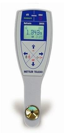
Calibration was performed by measuring the refractive indices of double-distilled water, toluene, cyclohexane, and carbon tetrachloride at defined temperature. The accuracy of the instrument is  $\pm 0.0005$ . 2-3 drops of the sample was put onto the measurement cell and the reading was taken. The refractive index of a sample depends on temperature. During measurement, refractometer determines the temperature and then corrects the refractive index to a temperature as desired by the user.
