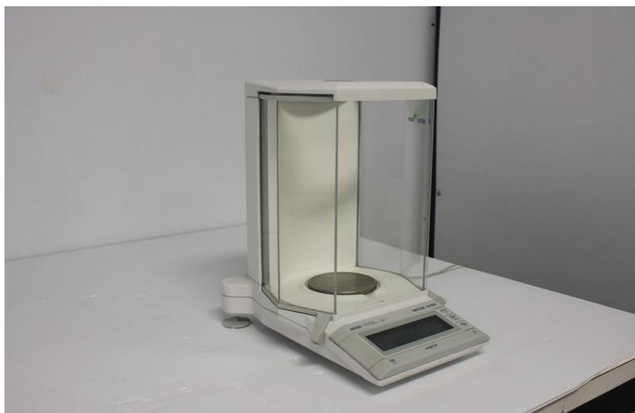
It can measure mass to a very high precision and accuracy. The weighing pan of a high precision (0.0001g) is inside a transparent enclosure with doors so that dust
