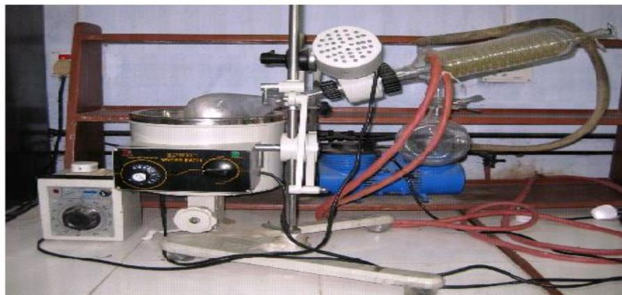
Rotary evaporation is most often and conveniently applied to separate "low boiling" solvents such as n-hexane or ethyl acetate from solid or mix compounds at atmospheric conditions. However, careful application also allows removal of a solvent from a sample containing a liquid compound if there and a sufficient diversity in boiling points at the selected temperature and reduced pressure.
