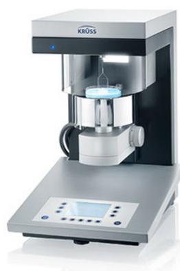
The surface tension experiments were completed by platinum ring detachment method using a Tensiometer (K9, KRÜSS; Germany) at the experimental temperature. The precision of the measurement was within  $\pm 0.1 \text{ mN}\cdot\text{m}^{-1}$ .
