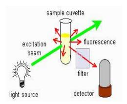
sample) and the emission spectrum (the light emitted by the sample) have been measured. The concentration of the analyte is directly proportional with the intensity of the emission.
