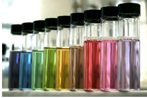
Figure 2.2 Nanoparticles of various shape and size in solution – the plasmonic resonance determines the colour.
