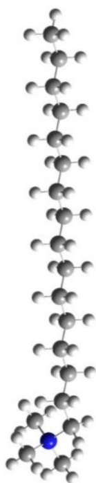
Figure-D.S2A. Optimized geometry at the B3LYP/6-31G level for isolated CTAB. Color code for atoms: blue, nitrogen; dark gray, carbon; and light gray, hydrogen
