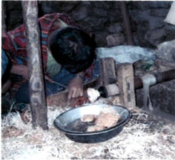
Indigenous entrepreneur curving a wooden bowl with his ancient but effective tool & technique. Oak roots serve as raw material for production of expensive wooden bowls.
