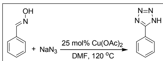
Scheme.III.A.6. Copper acetate catalyzed synthesis of 5-substituted 1 H -tetrazoles from various oximes and sodium azide
