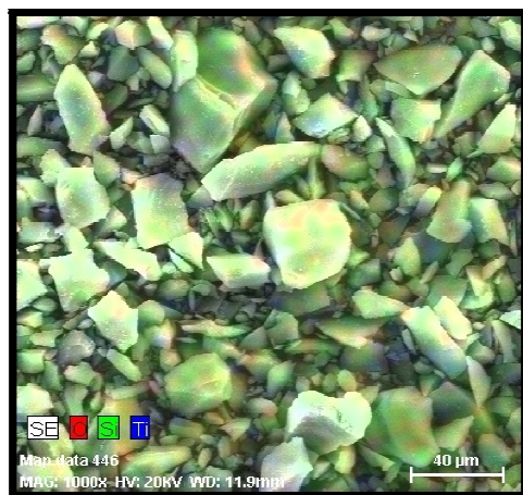
Fig.VI.B.15. Elemental mapping of titanium-silica after fifth reaction run
