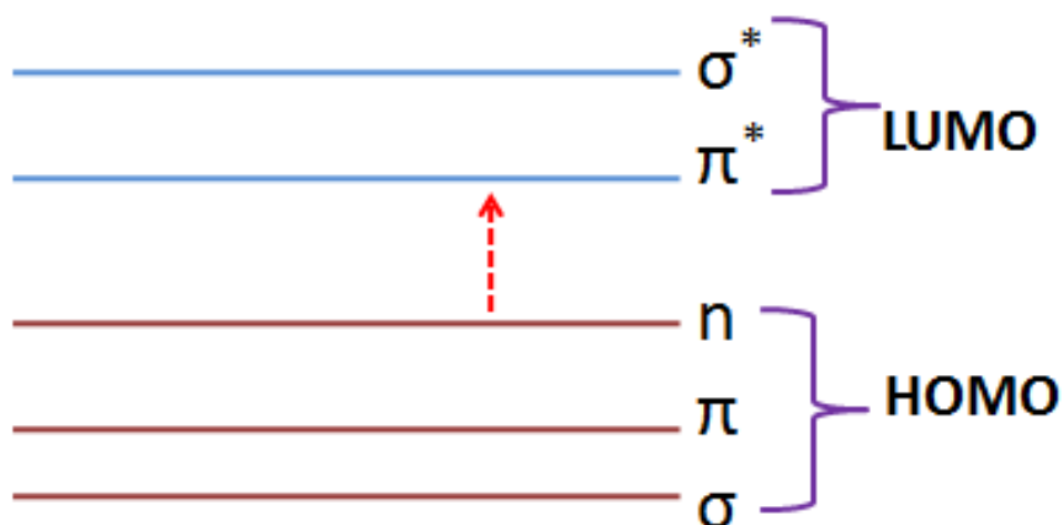
Figure 5.5 Possible transition mechanism in the Rose Bengal molecular system.
