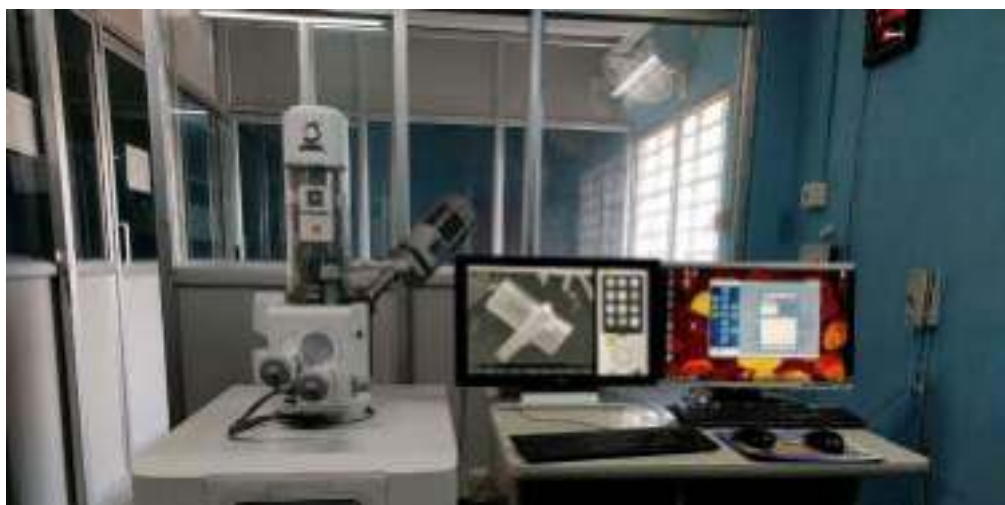
Figure 2.3 Experimental setup for SEM and EDS measurement.
