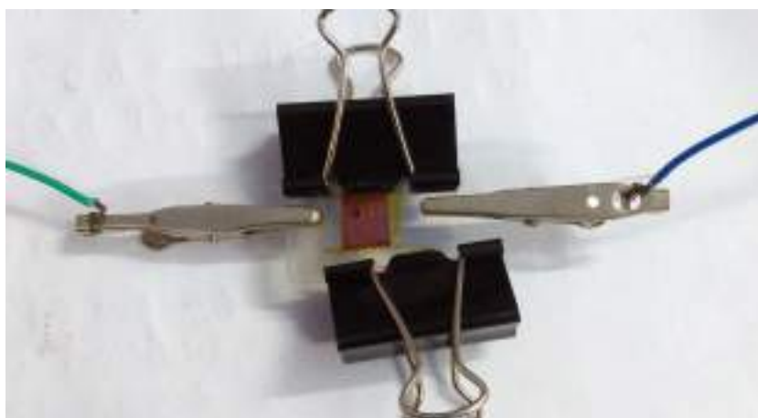
Figure 4.3 DSSC fabricated with N3 dye and \text{WO}_3 as photoanode material.
