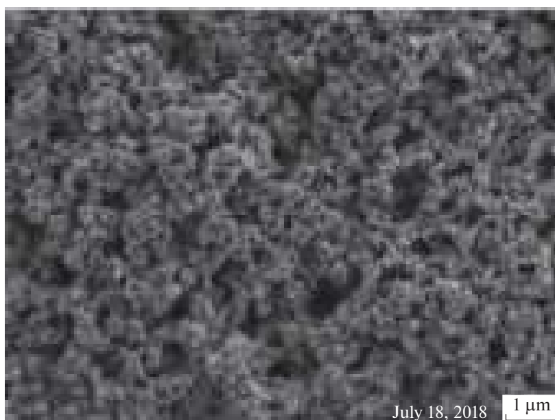
Fig. 3. Scanning electron microscope (SEM) image of \text{TiO}_2 nanoparticles on FTO substrate.
